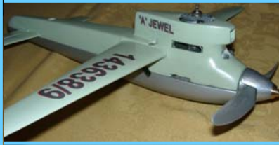
[Above right] Geoff and Harry Walker's first venture into Speed (following Geoff's retirement from active Team Racing) was this Sadler "Little Rocket" with Super Tigre G31 1.5 cc diesel. For their second, [above left] it's a G20 glow powered "A Jewel", Larry Grogan's US Nats winner.
