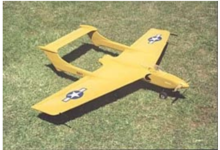
John Goodge's "Sea Vixen / OS 46 LA" - Note the extended lead-out guide on the inboard wingtip to cater for the very sharp sweep-back.
