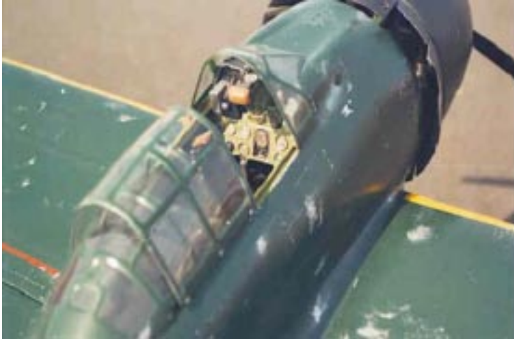
A photo from Ron Burn, showing the cockpit detail of his Japanese 'Zero' stunter. Note the careful weathering of the paint to give the appearance of an aircraft that has been in use.
