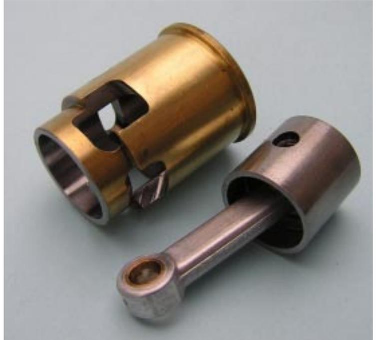
*"Thick cylinder wall doubles as upper transfers, adds stiffness."*
