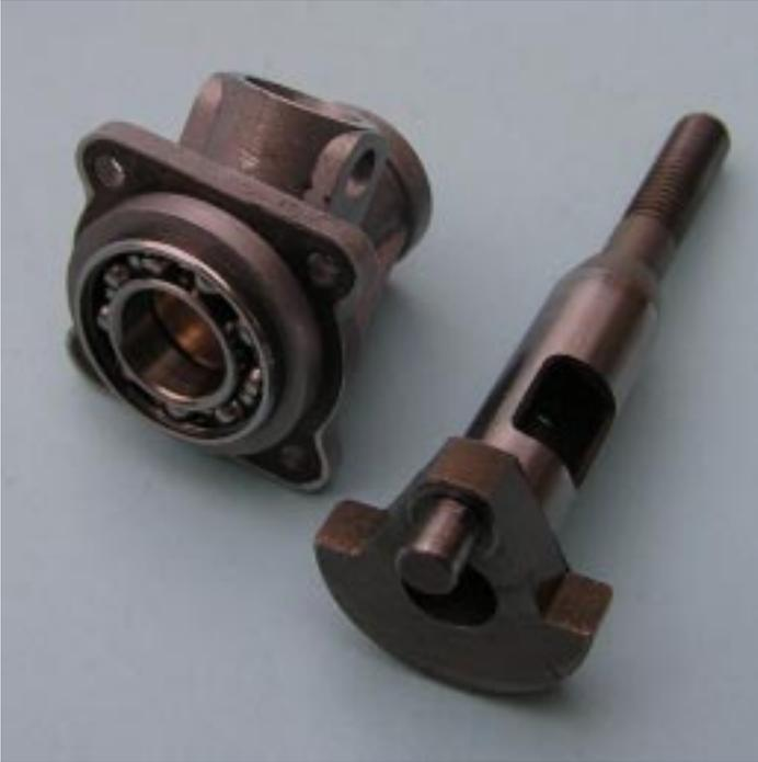
*“Well balanced crankshaft rides in rear bearing. Only front few millimetres touch bronze bushing.”*
