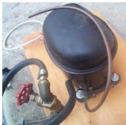
Fridge Vacuum Pump. Copper pipe is "blow". Rubber is "suck".
