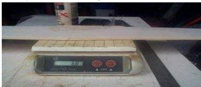
Wing before "bagging", 68 grams. After 80 grams.
