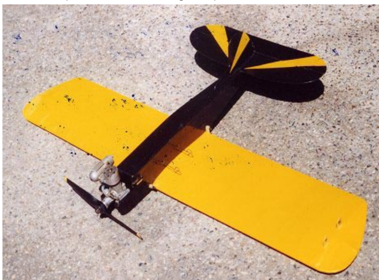
APS Juggler design circa 1950. photo from Alwyn Smith. It has an OS Max .25 and Master 9 x 4 prop. This design was very popular in the early 1950s, usually powered by Frog 500 (.29 cu in.) engines. (For more on this see Ray Sherburn's comments in the TARMAC notes for April & May last year.)
