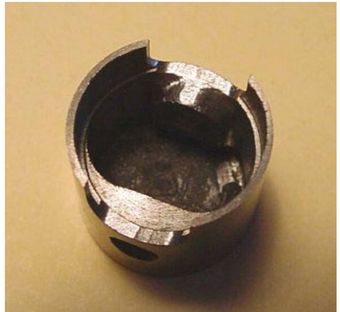
The reworked piston with thinner, notched skirt and one lightened gudgeon boss completed.
