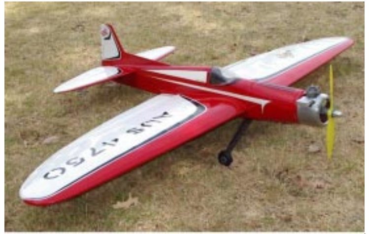
Thunderbird. The outstanding finish is in automotive acrylic with a two pack clearcoat over the top. As one of the bystanders said at it's first outing 'That paint job is going to be a hard act to follow' The finished weight is 42 and a bit ounces and the model is powered by an Aldrich prepared Veco .35 just like Bob Palmer's original.
