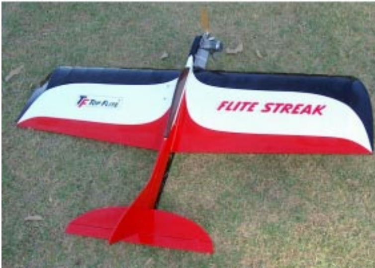
Jim Trevaskis' freshly finished TopFlite ARF 'Flite Streak. This one is powered with an OS .25
