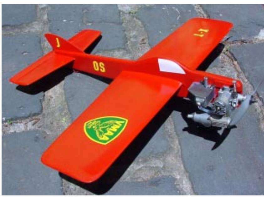
This trainer model which was built by John Hallowell was recently successfully test flown at Doncaster “John can't help himself....reckons the new model should be good for 50 laps at 20/10” Note hopper tank to help maintain feed when novice gets model into free flight.
