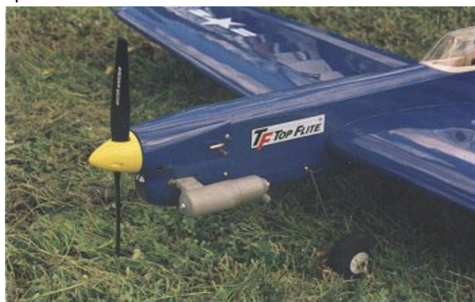
Photo above: The cowl overlaying the top and sides of the fuselage. The two small pipes are the remote tank vents.
