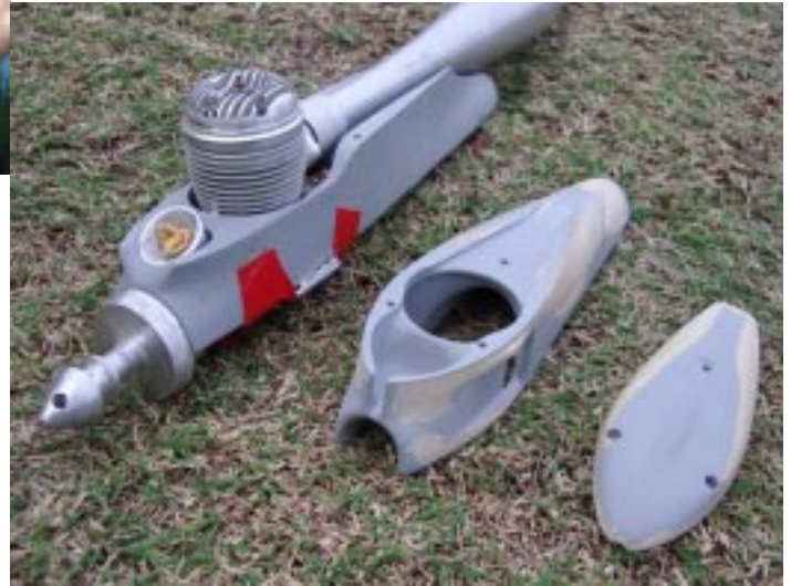
Here is a shot of the three separate parts of Grant's patterns for the ducted speed model cowl. All the cooling air for the head will enter the front plenum chamber where it will have the cooling mist introduced (from a pressurised tank behind the cylinder).
