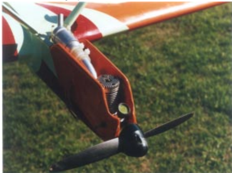
Exhaust layout shows the 3 fixings and the way the plastic joining tube counters the engine off-set.
