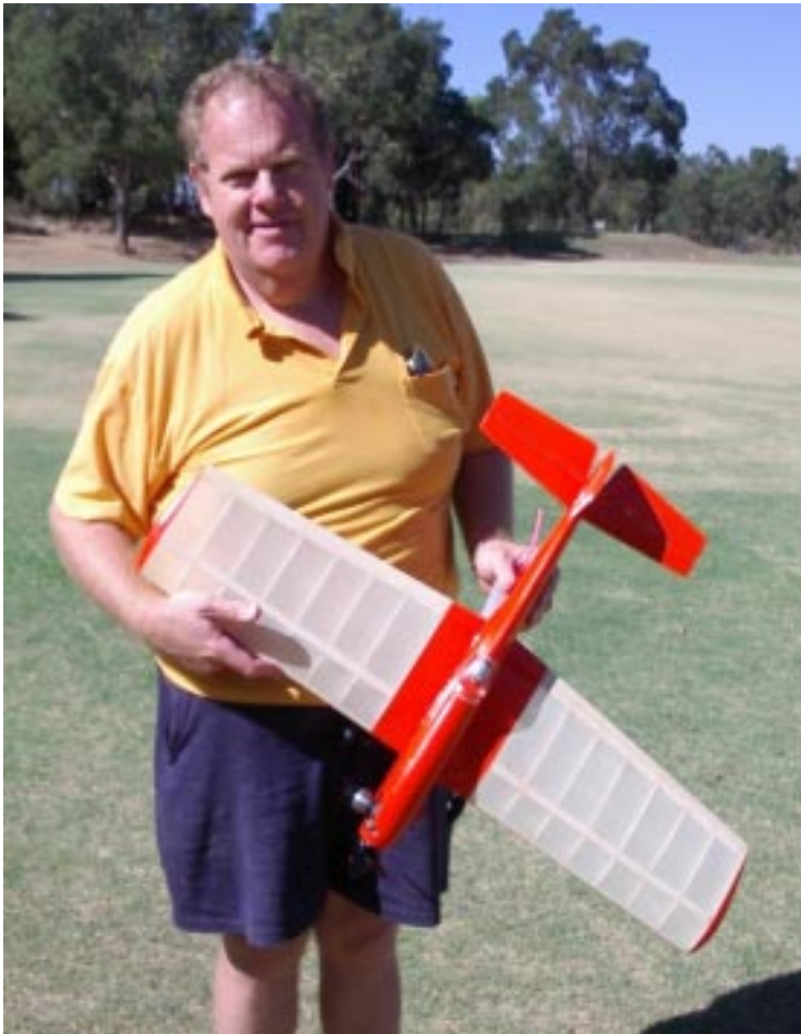
Smiling Fred Adler and his latest vintage stunt model. It is an 'Ambassador' built from Aeromodeller plans. Silk covered and powered by a rare Gordon Burford 'Sabre .15' 2.5cc diesel engine.
