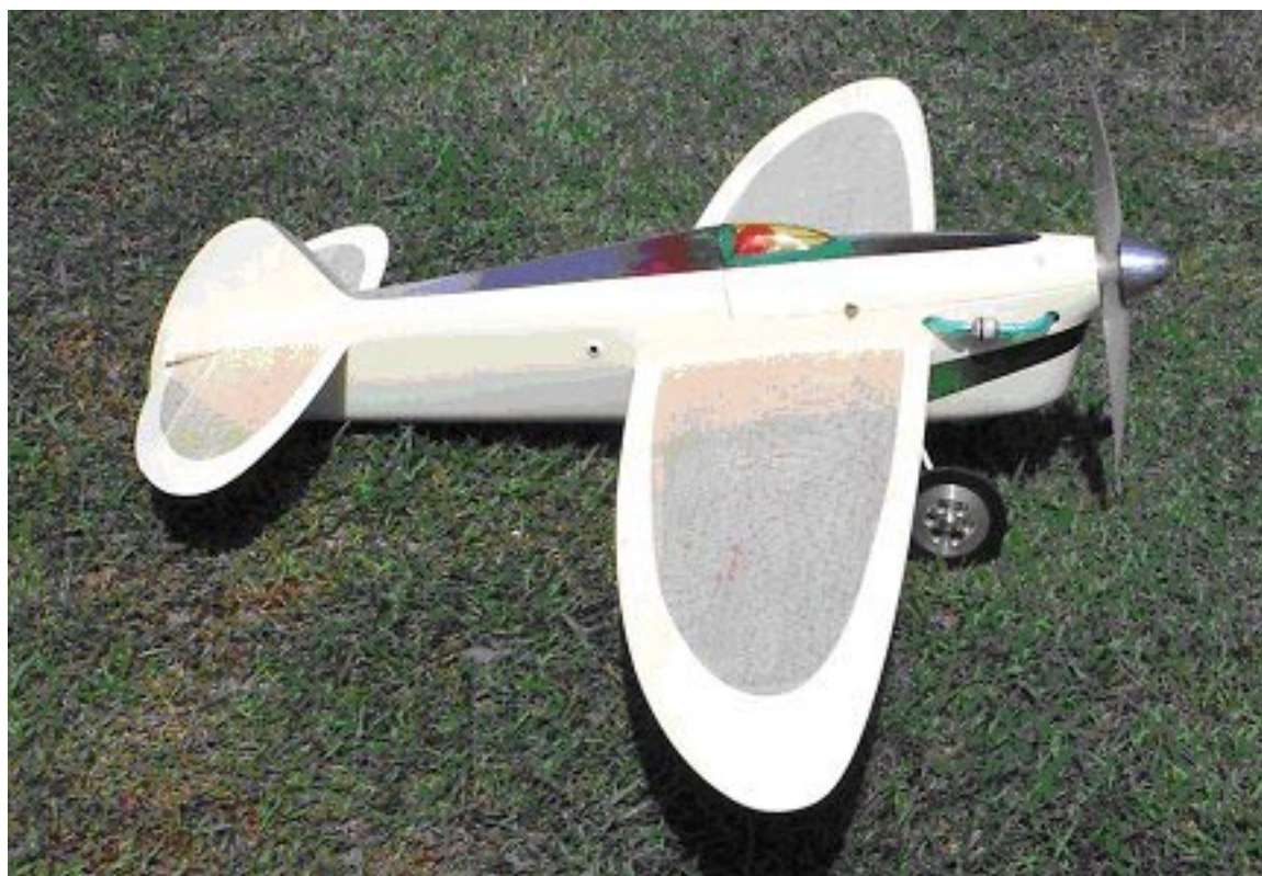
Here is Mark McDermott's new Classic B team racer. It is a 'Galaxie' powered by an OS .25 and as can be seen has a very high gloss finish.
