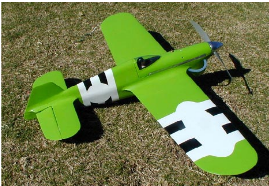
A new Classic B racer built by Mark Sherburn. A sort of enlarged and modified VooDoo powered by OS .25. I think that the engine has been breathed on by Darryl Mills. It looks good and is in the process of being race tuned now. The photo by Adrian Dyson.
