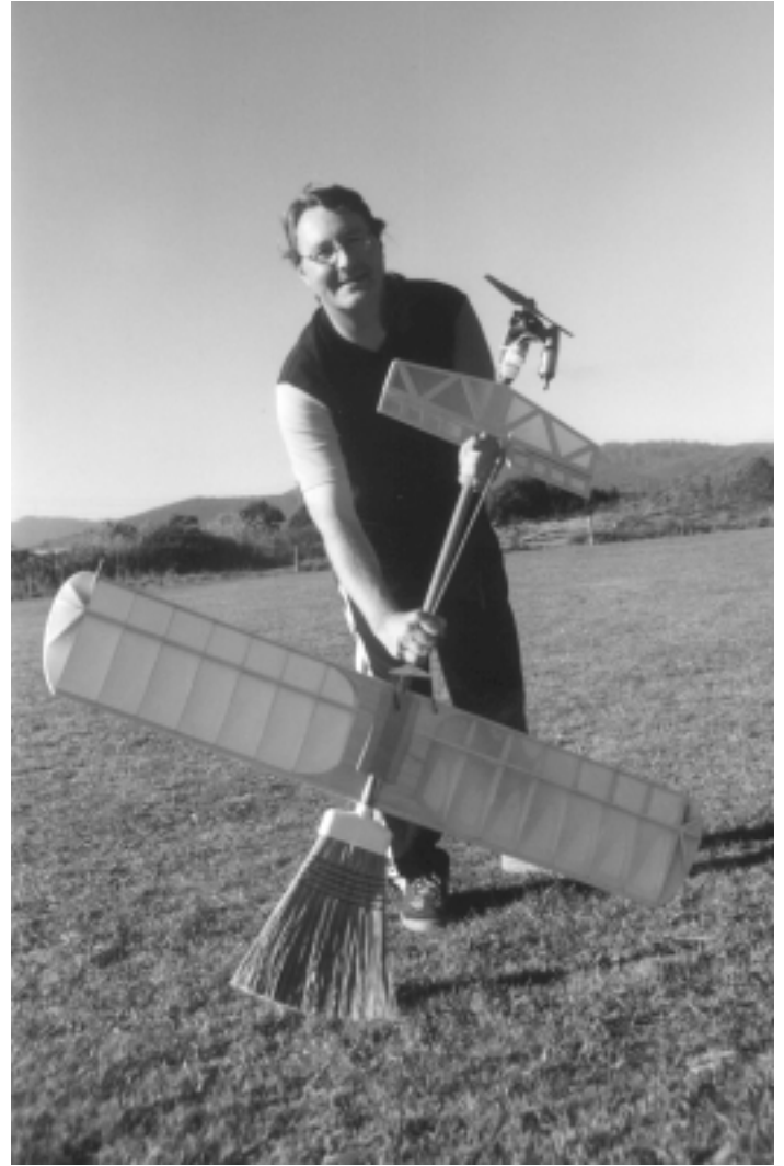
Ken Taylor's latest model, called Krystal, is a 63 inch stunter powered by his MVVS49. This one has a very thick wing and is reasonably light.
