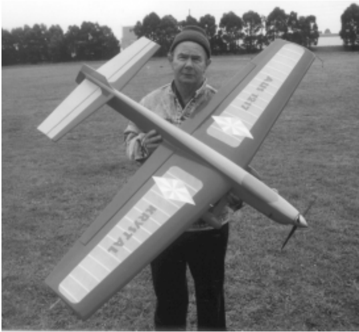
Ken Taylor's latest model, called Krystal, is a 63 inch stunter powered by his MVVS49. This one has a very thick wing and is reasonably light.
