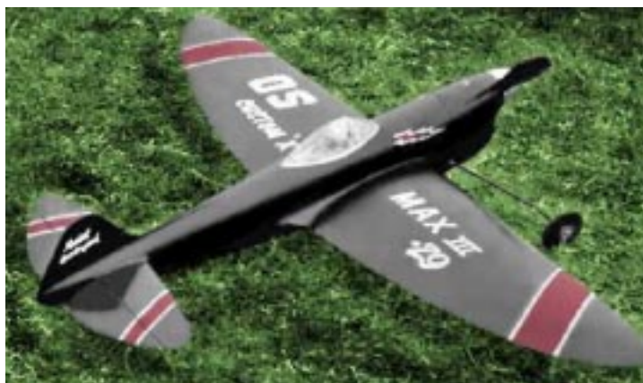
Pic. 2. Tony Farnan's second placed Kanga team racer is capable of speeds over 100 mph.
