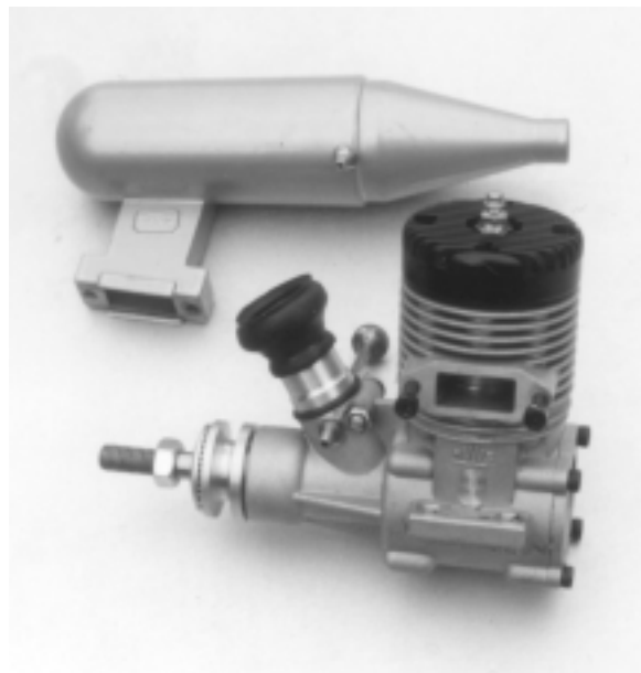
MVVS 49 Stunt as tested with the conventional side exhaust and front needle.
