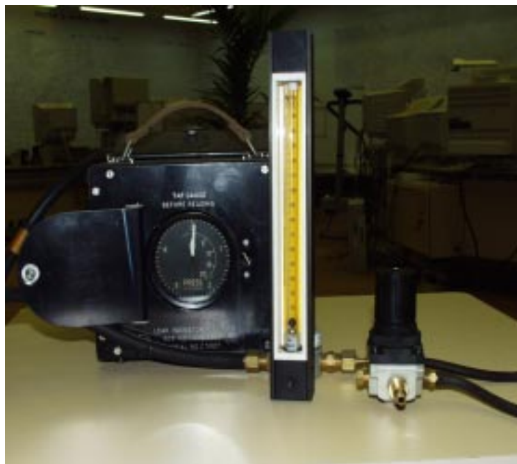
Above :- Flow testing Rotameter used for calibrating metering jets.
