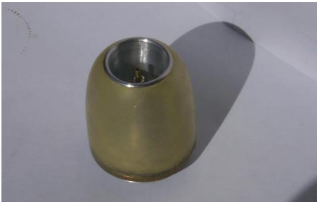
Tuned intake and cowl as a complete head. (not a detailed photo)
