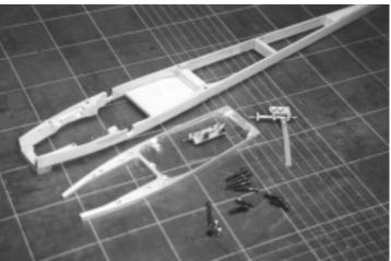
Disassembled pan, crutch, shutoff and remote NVA Wings (Completed since photos) are 6mm + 3mm balsa, finished all over with epoxy and 1/2 ounce glass.
