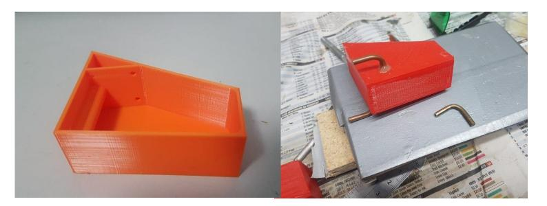
The above pictures of the internal of the tank show the front feed and baffle, the finished tank, 90 degree bends of tubing glued in with cyano and small slow set epoxy seal for added measure.
