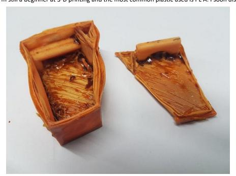
This is the result of glow fuel in the first PLA tank. The dark bits are the remains of finishing epoxy which I used in an attempt to seal the tank.
