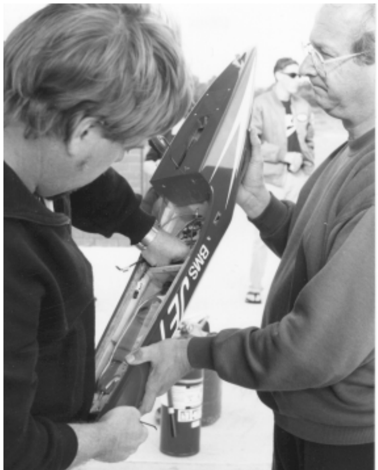
Bob Fry (Left) and Alisdair Taylor replace the burst fuel tank before the first flight.
