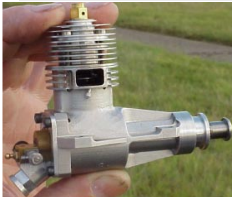
Above:- Brian Turner's (U.K.) handmade F2C engine. Brian makes all the components including the crankcase which is machined from a solid billet of special aluminium alloy
