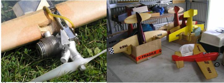
Murray Wilson had modified the plumbing on his Half A combat model. The inboard mounted vent completely eliminated a misfire that had been taking place during flight manoeuvres.
