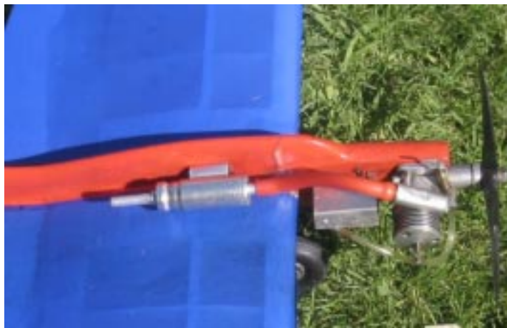
Above :- Silencer fitted to a PAW 2.49 in a Peacemaker.
